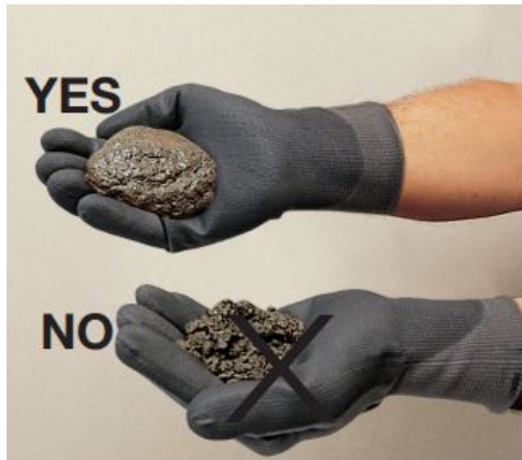
The correct consistency of Mapecem
