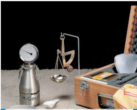
Carbide hygrometer for measuring the moisture level of a Mapecem screed
